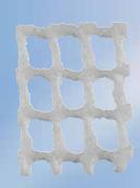
After 90 days it is clearly seen that a major part of the material has disintegrated. On the left is an original piece of X-LITE® and to the right the same piece after 90 days composted.
